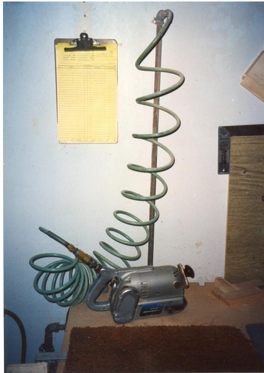
A pneumatically powered belt sander lies on a workbench in an Amish carpentry shop.
